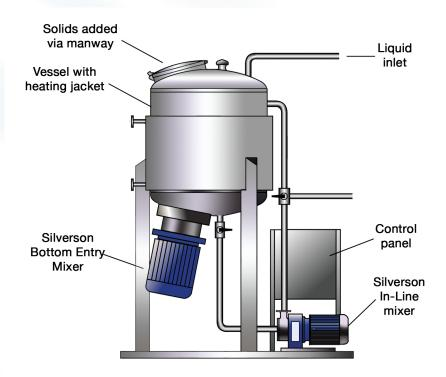
In a typical operating procedure the vessel is first charged with the base fluid, most commonly water. This is heated to the required working temperature before the Bottom Entry mixer is started and the product for reclaim is added. Large solids can be added without the need for pre-grinding. The mixer exerts a powerful suction which draws the materials down into the workhead, where they are rapidly reduced to granular size.
