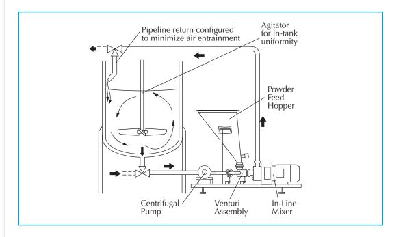
The base liquid is drawn from the vessel by the centrifugal pump and passed through the venturi assembly into the In-Line Mixer. The high velocity flow through the venturi creates a vacuum in the chamber below the powder hopper. The liquid is returned to the vessel by the self-pumping In-Line Mixer.
