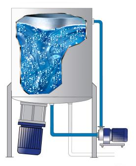
Once the solids have been reduced to granular size the Silverson In-Line mixer is started. The product is drawn from the vessel and processed in the rotor/stator workhead of the In-Line mixer before being returned to the vessel by the self pumping action of the In-Line mixer.
