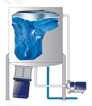
The intense high shear exerted on the polymer by the bottom entry and In-Line mixers ensures that particle size is minimized, exposing a greater surface area of polymer to the surrounding oil, allowing rapid solubilization to be achieved. Samples can be drawn off to check dispersion and solubilization is complete before the finished product is discharged.
