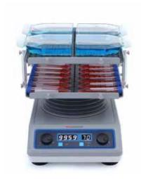
Digital Platform Rocker with Double-Tier Platform attached (flasks and containers sold separately).
